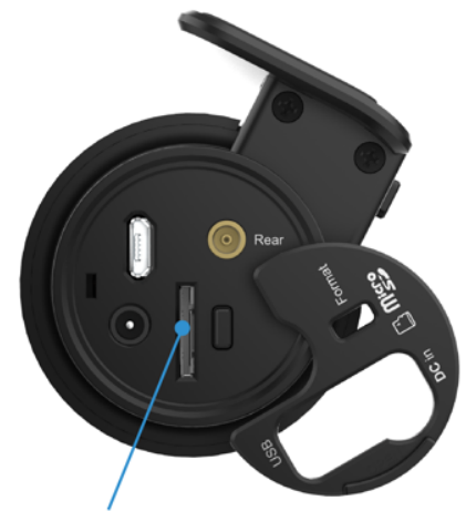
MICROSD CARD SLOT Unplug the power cable to open the cover
