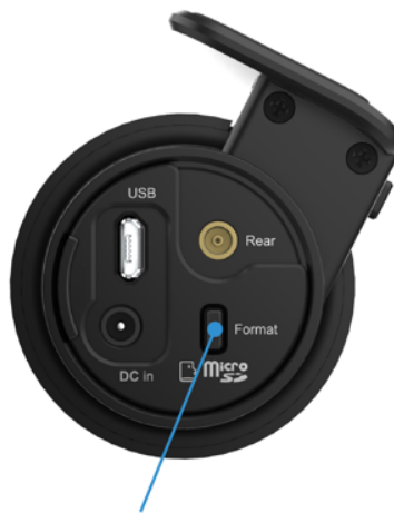
FORMAT BUTTON to format the microSD Card
